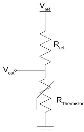
Additional length may be spliced to the cable without adverse consequence. The series resistance of the cable extension adds minimal resistance when compared to the thermistor resistance value. 1000 ft of 20 AWG wire only adds about 10 ohms, less than 0.2% of the thermistor resistance at 105°C. At lower temperatures and in most applications, the added resistance of an extension cable can be ignored.
