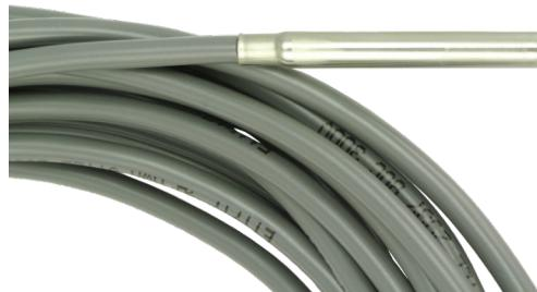
Unlike thermistors that are simply potted in simple straight tubes, the swaged stainless steel tube used for TSSP-1 will not come off in cyclic temperature environments.
